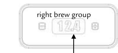
Temperature display steam boiler (t2, here 124°C) dot in the 2 nd position
